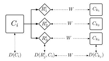
**Fig. 2.** Compositional cases consist of a complex component  $C_i$  that specifies the roles for the required subcomponents  $(R_j^i)$  and the bindings (W) of those roles with further components  $(C_{k_j})$ . Compositional cases and roles have descriptions (D) used to establish valid matchings in the application domain.
