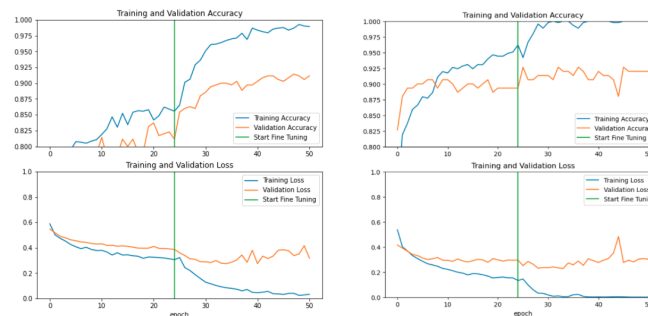
Figure 7. The comparison of model training performances between Majority Voting (left) and Dawid-Skene (right) consensus training datasets.
