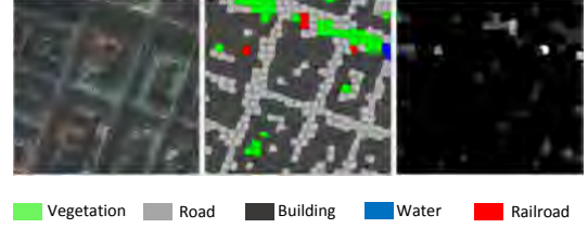
Figure 4: Left: Input RGB image together with the segmentation. Middle: Classified segmentation from the classifier. Right: Average reconstruction error for each segment where bright areas indicate suspected classification errors.
