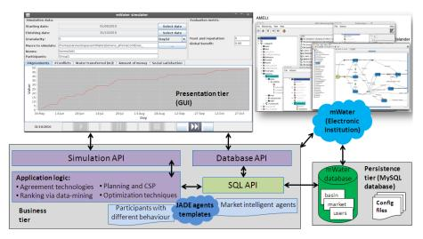
Fig. 1.6 Multi-tier architecture of the *mWater* system
