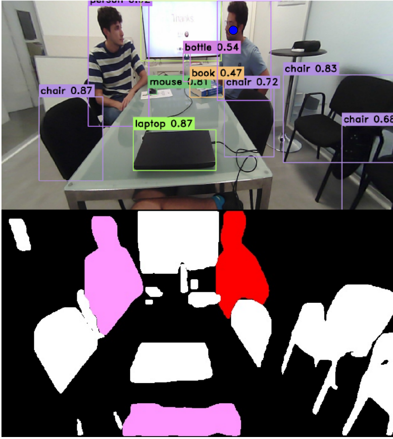
Fig. 2. In the upper image, the results of the object detection for one of the task frames. The blue dot represents the estimated gazing point of the participant. In the lower image, the looked-at segmentation mask is highlighted.
