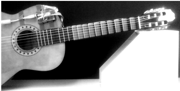
Figure 1: Gesture caption system based on capacitive sensors (mounted on the fretboard) and Arduino (mounted on the body).
