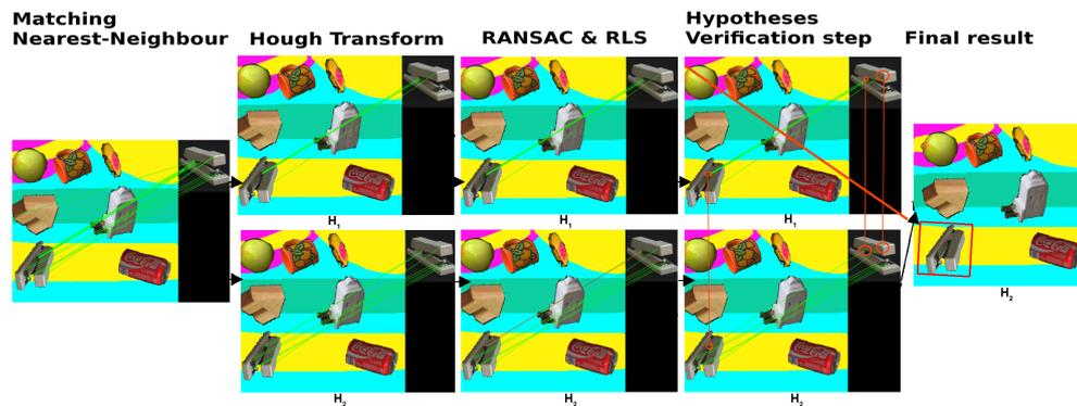
Figure 2. Example of execution where the final hypotheses verification step detects two hypotheses that refers to the same object instance
