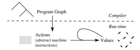
Figure 6: The Sartor architecture. The compiler protocol translates the source program graph into actions, or abstract machine instructions. The runtime protocol executes those actions, producing and operating on runtime data objects.
